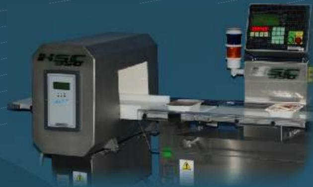
The contaminated product can be expelled with a dedicated ejector and accumulated "under key", in accordance with the alimentary packaging norms in force.
