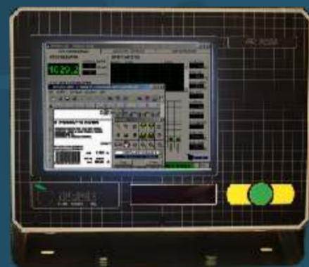
The 8" touch screen, applicable on the entire HSC350 model range, is provided with Wireless or Bluetooth connection and external infrared keyboard with trackball; with the execution of Windows™ tasks, it allows an easy integration of different printers and a client-side connection with plant database.
